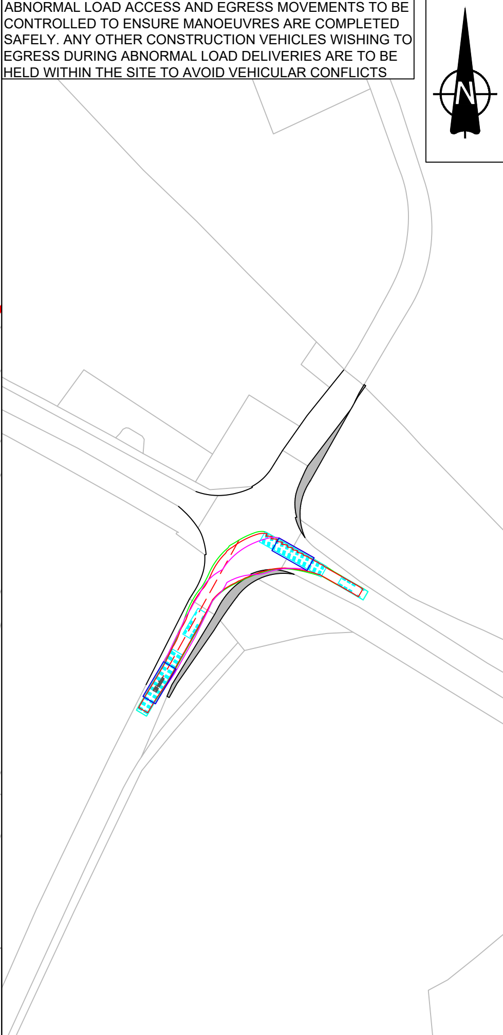
INSET C: 31m 132kV TRANSFORMER VEHICLE RIGHT TURN ONTO PENNY HILL LANE - SCALE 1:1000
